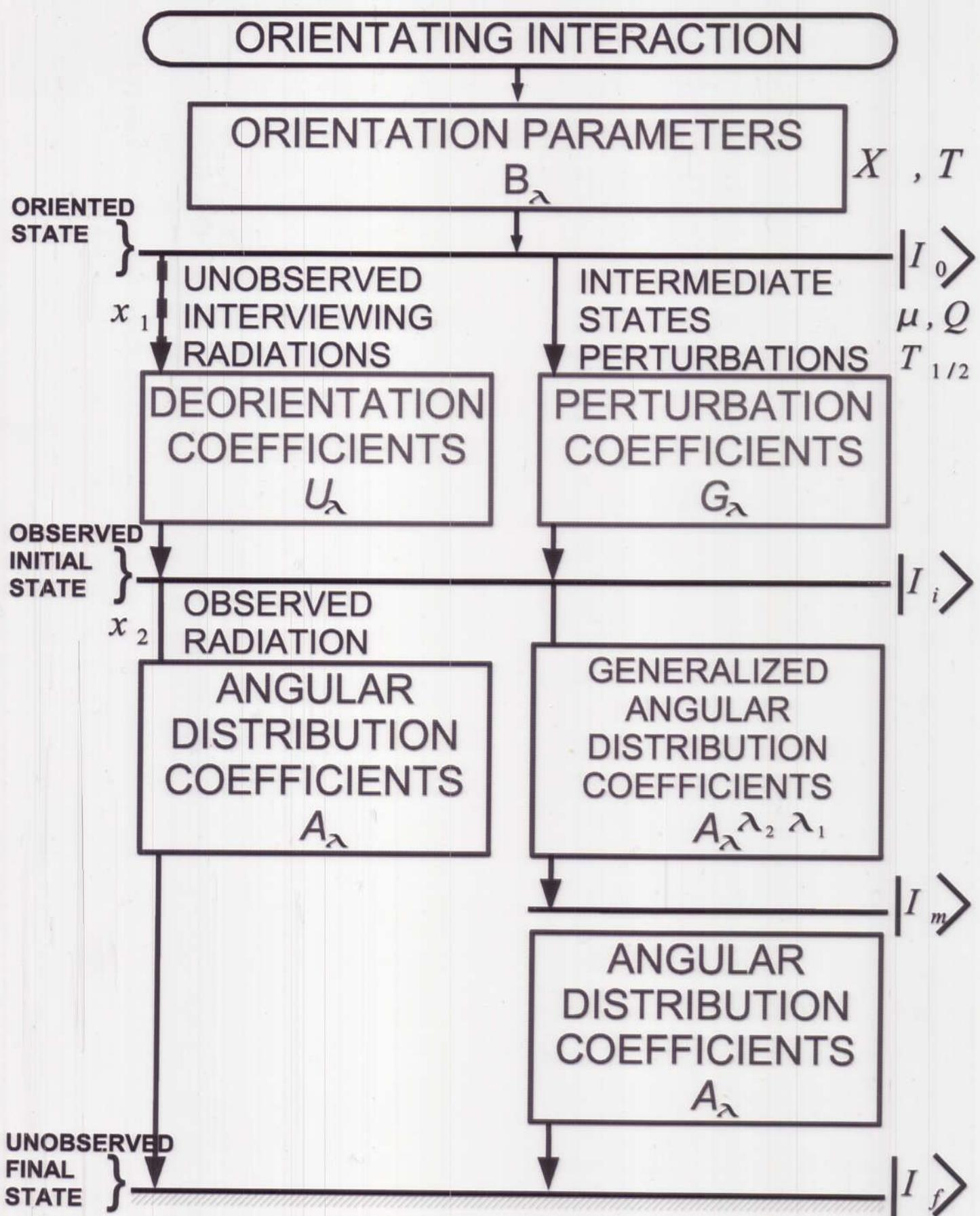
$$W_{x_2}(\theta, \varphi, T, t) = \sum_{\lambda} B_{\lambda}(X, T, I_0 \mu, Q) \cdot U_{\lambda}[I_0 I_i (LL' \lambda)_{x_1}] \cdot A_{\lambda}[I_i I_f (LL' \delta)_{x_2}] \cdot Q_{\lambda} \cdot P_{\lambda}(\cos \theta)$$
