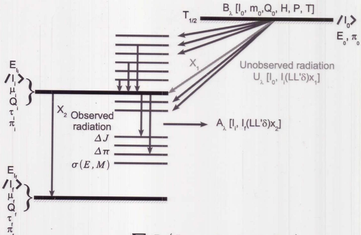
$$W_{x_2}(\theta, \varphi, T, t) = \sum_{\lambda} B_{\lambda}(I_0, \mu_0, Q_0, H, P, T, t) \cdot U_{\lambda}[I_0 I_i(LL'\lambda)_{x_1}] \cdot A[I_i I_f(LL'\delta)_{x_2}] \cdot Q_{\lambda} \cdot G_{\lambda} \cdot P(\cos \theta)$$
