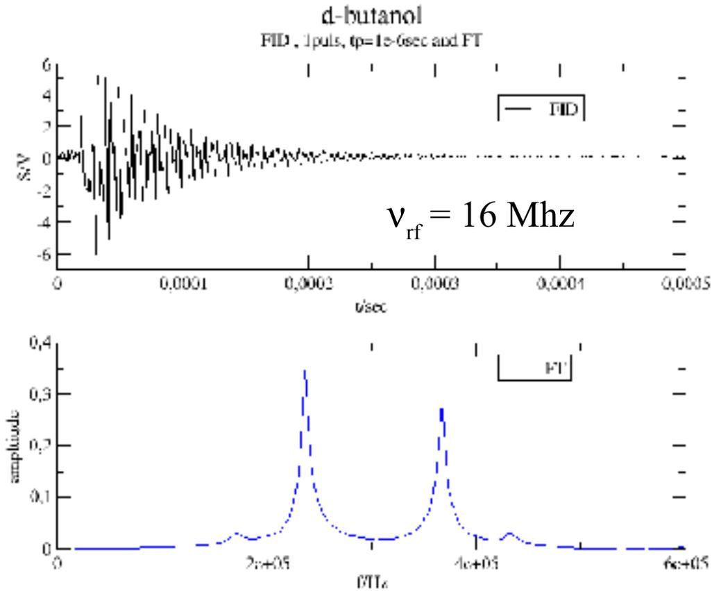
A finite time after the pulse the preamplifier is saturated and the detected FID is unusable, but the whole FID must be Fourier transformed to optaine the complete line shape.
