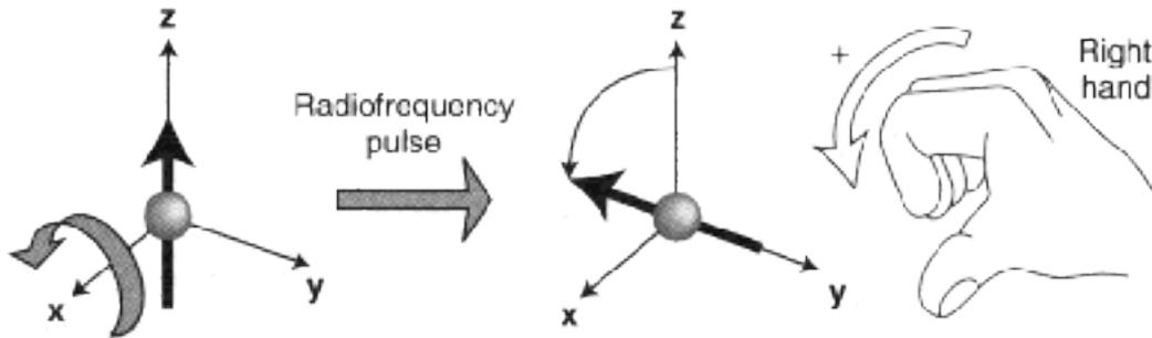
By applying a rf pulse every signal spin is rotated by  $\pi/2$  about the  $x$ -axis.
