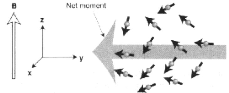
Since the pulse rotates the polarization of every spin the net polarization is therefore transformed along the  $-y$ -axis; thus a *transverse magnetization* arises.
