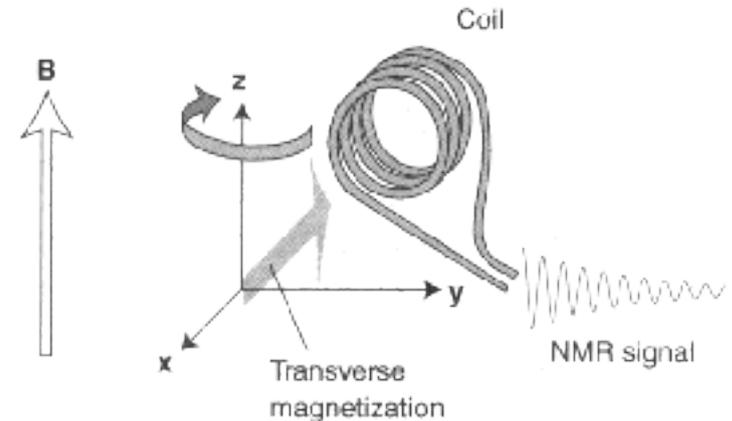
The rotating net magnetic moment induces an oscillating signal in the receiver coil
