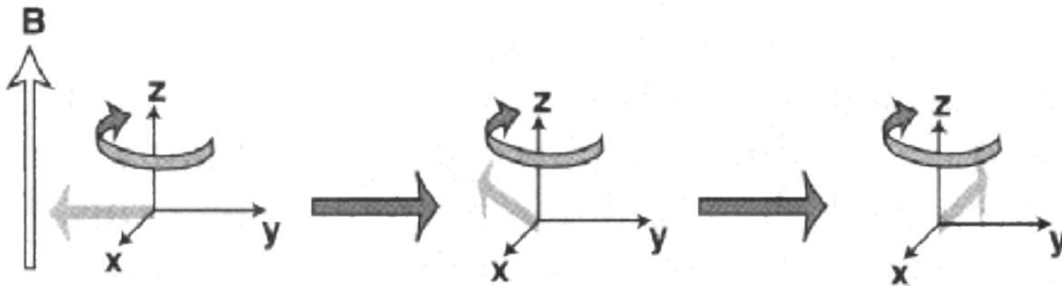
Because every signal spin starts its precession motion, the transverse magnetization also precesses in the  $xy$ -plane, perpendicular to the magnetic field.
