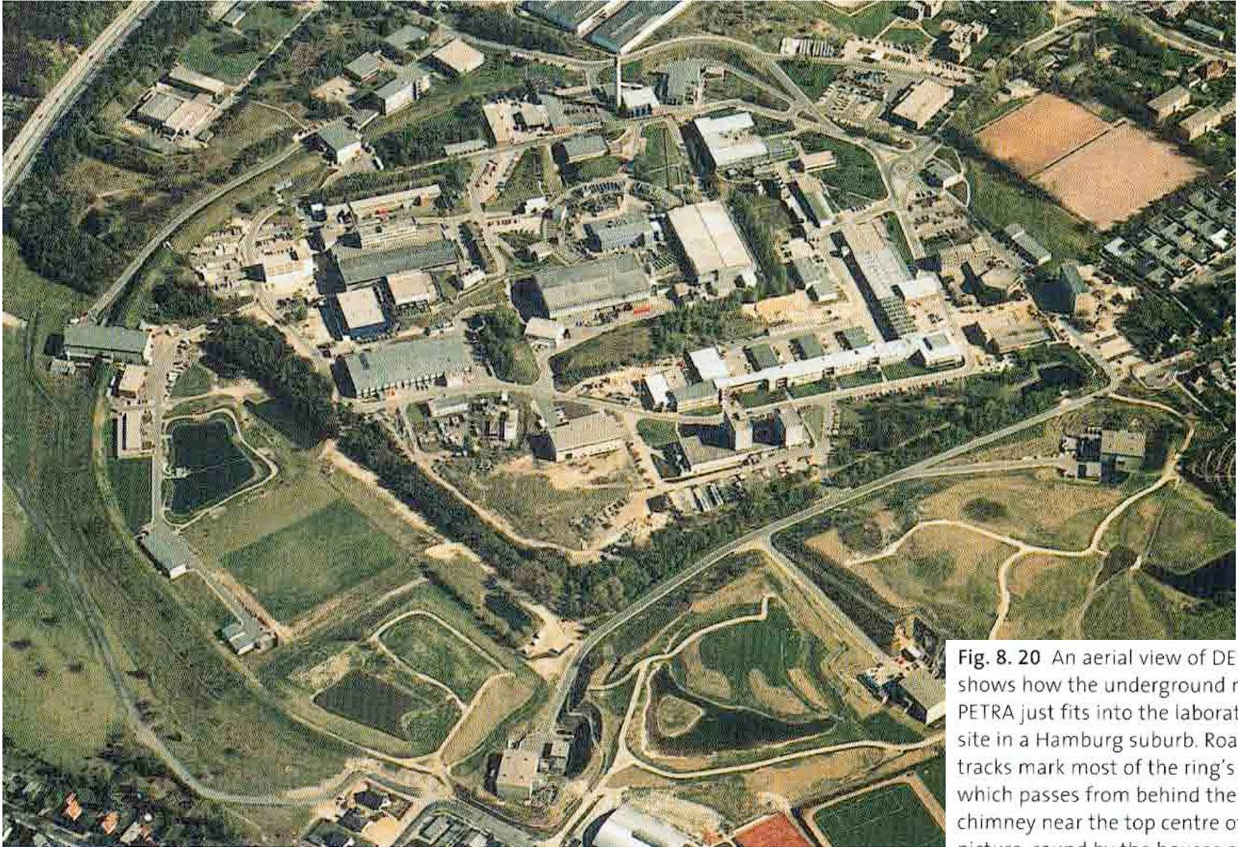
**Fig. 8. 20** An aerial view of DESY shows how the underground ring for PETRA just fits into the laboratory's site in a Hamburg suburb. Roads and tracks mark most of the ring's path, which passes from behind the chimney near the top centre of the picture, round by the houses at the right, close to the sports field at the bottom, and back up across the fields at the left.
