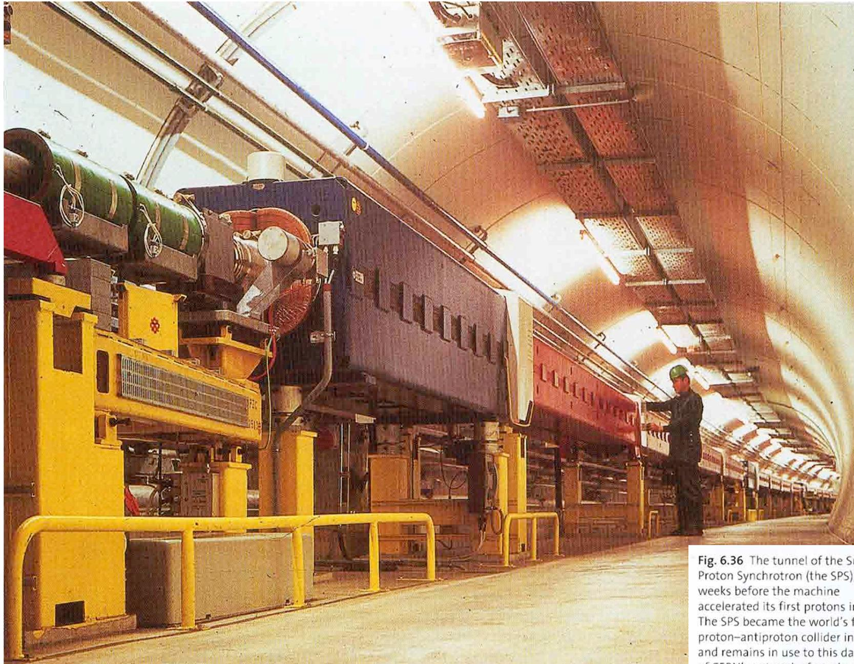
Fig. 6.36 The tunnel of the Super Proton Synchrotron (the SPS), in the weeks before the machine accelerated its first protons in 1976. The SPS became the world's first proton-antiproton collider in 1981, and remains in use to this day as part of CERN's network of accelerators.
