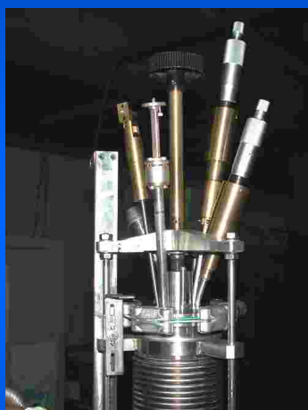
Head of ESR insert with mirror and coupling pin adjustment
