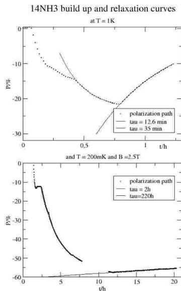
Measured at 2 different temperatures:
