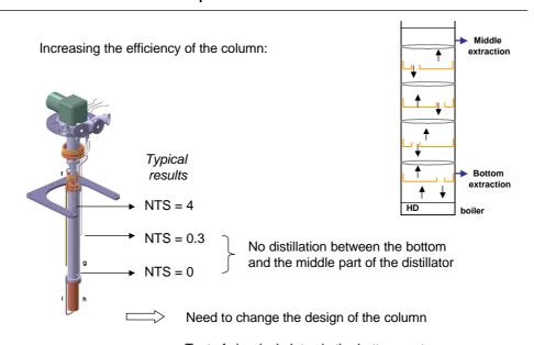
Test of classical plates in the bottom part to retain more liquid in the column
