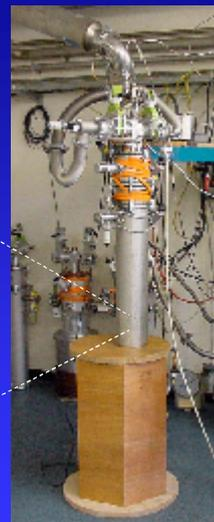
Standard PSI Laboratory Cryostat
