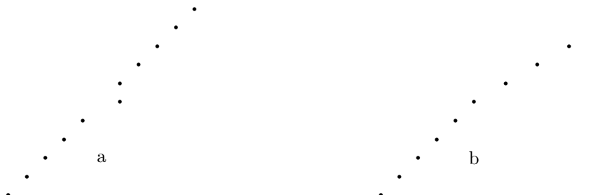
Figure 7: Two causes of bad track fits. (a) shows a track with one bad point, and (b) shows a track that will be split into two tracks.
