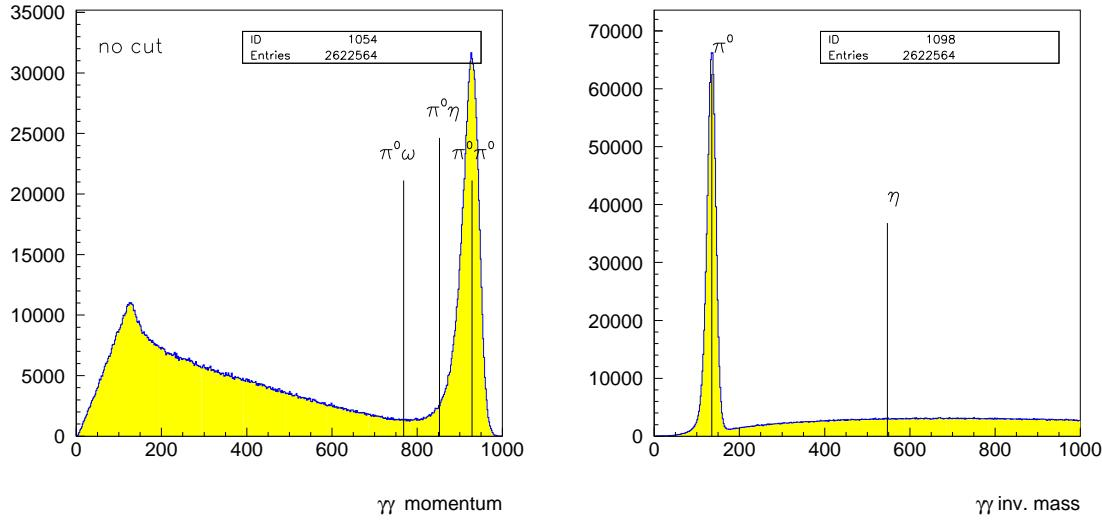
Figure 2.11: (left) Momentum of all  $2\pi^0$ 's. Each  $\pi^0\pi^0$  events causes two entries in the peak on the right side.
