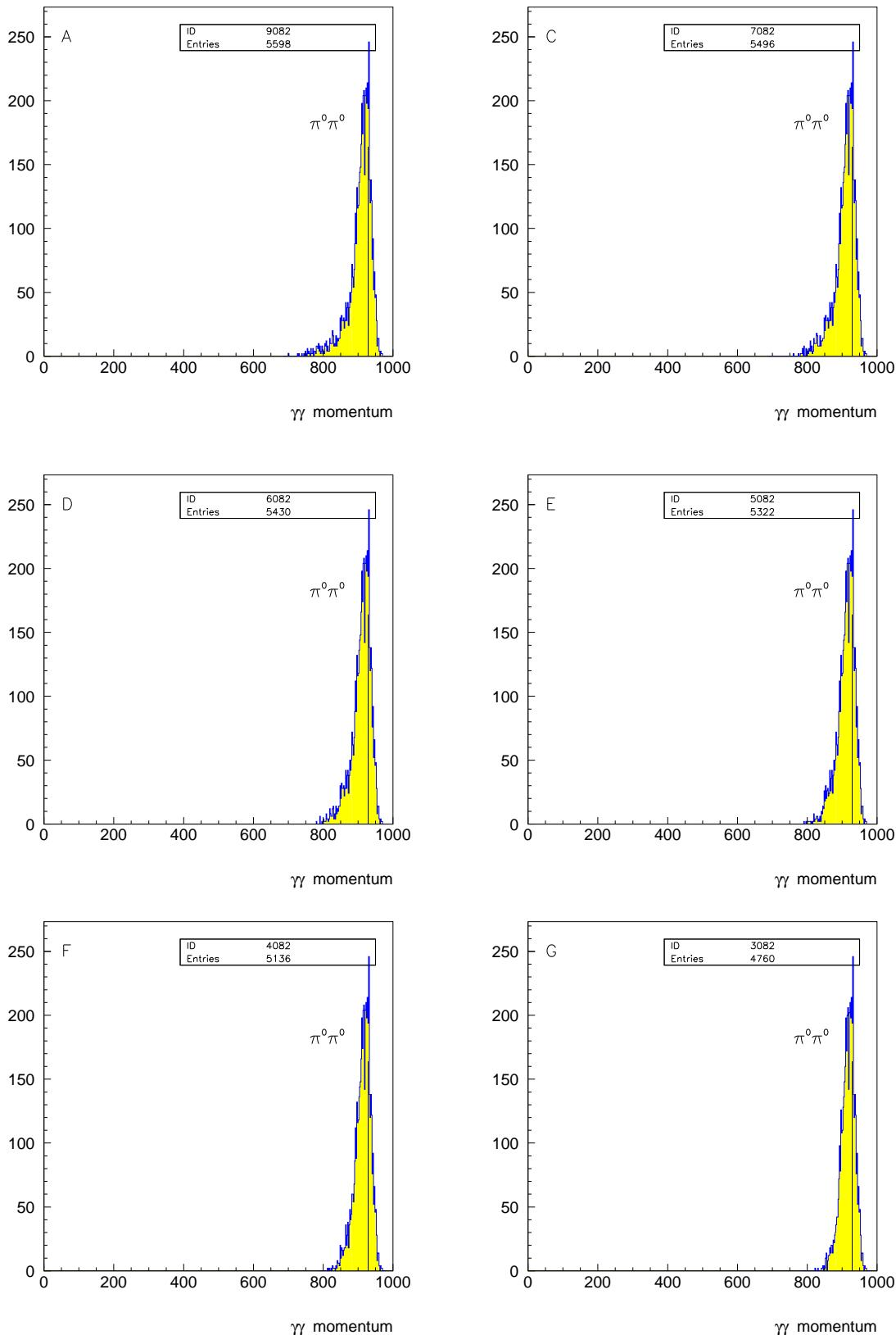
Figure 2.5: Momentum of  $\pi^0$ 's for  $\pi^0\pi^0$  final state. The letters are referring to the kinematical regions listed in report [1].
