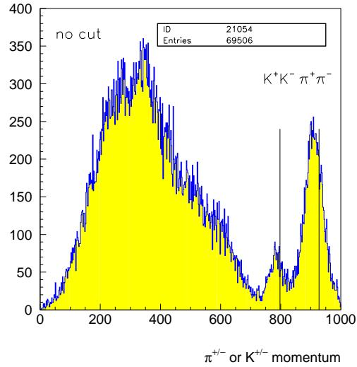
Figure 3.1: Momentum of two prongs. Each event causes two entry.
