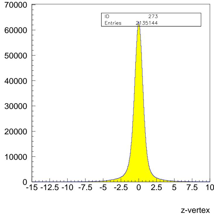
Figure 1.1: Vertex  $z$  distribution for charged tracks.
